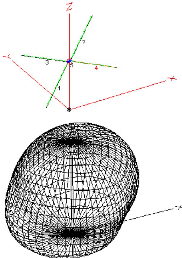
**Figure 9: Cross-Dipole Antenna Pattern at 40m**
