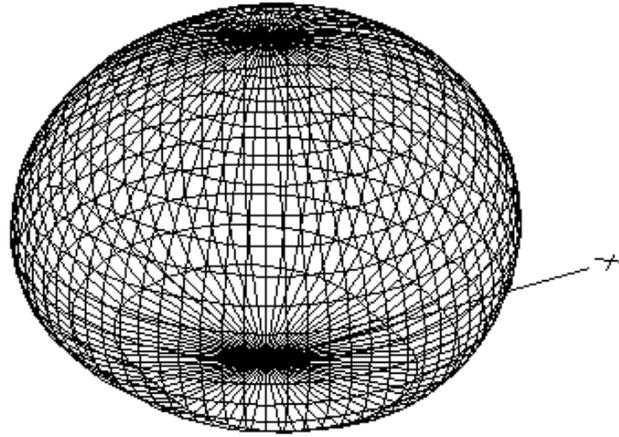
**Figure 11: 75m Inverted-V NVIS Antenna at 3.75 MHz**
