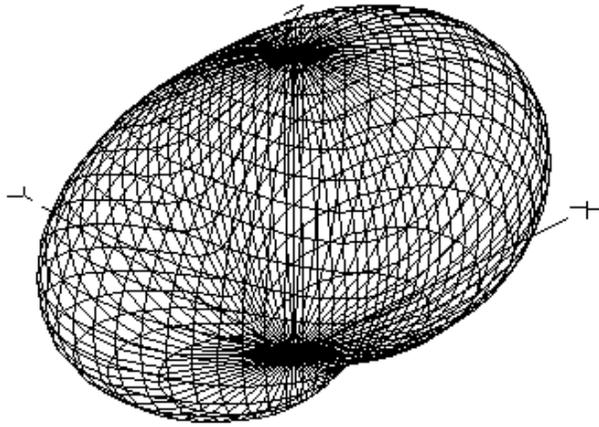
**Figure 8: 75m NVIS Dipole Pattern at 40m**
