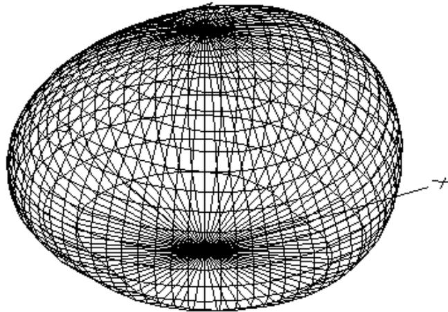
**Figure 12: 75m Inverted-V NVIS Antenna at 7.2 MHz**
