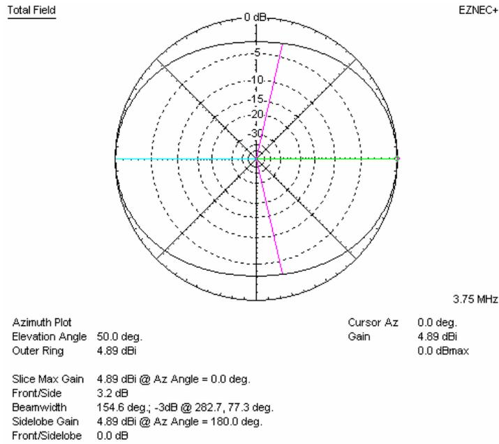
**Figure 3: Azimuth Pattern NVIS 75m Dipole**
