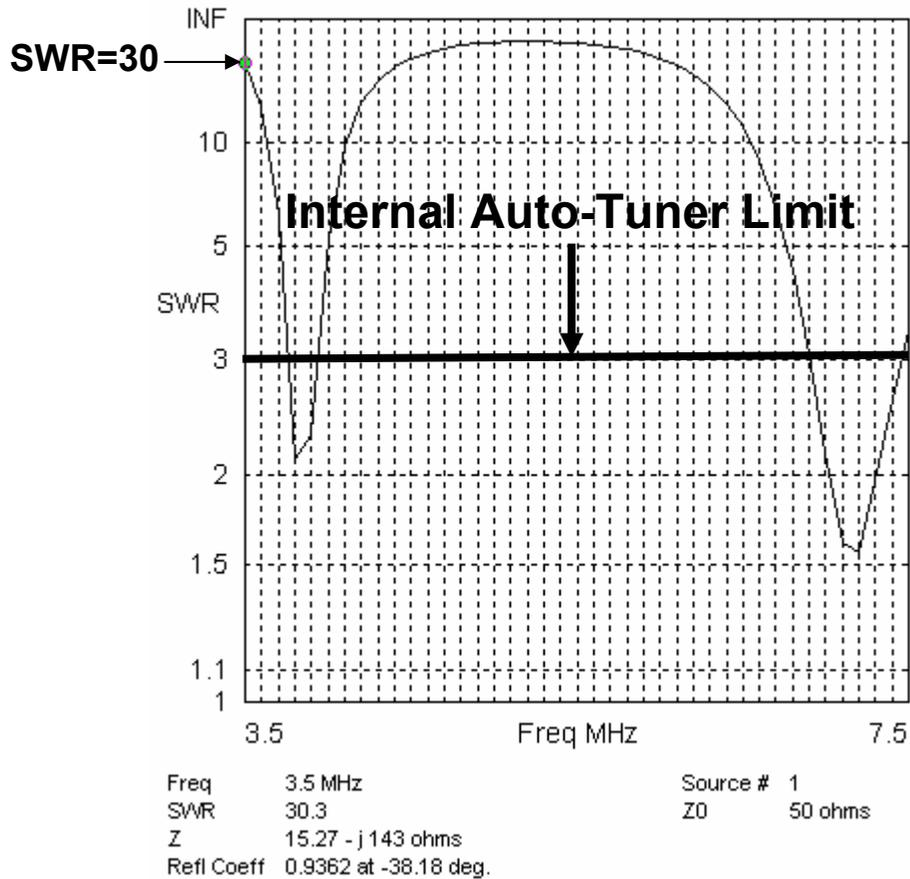
**Figure 14: SWR Plot of Cross-Dipole NVIS Antenna**
