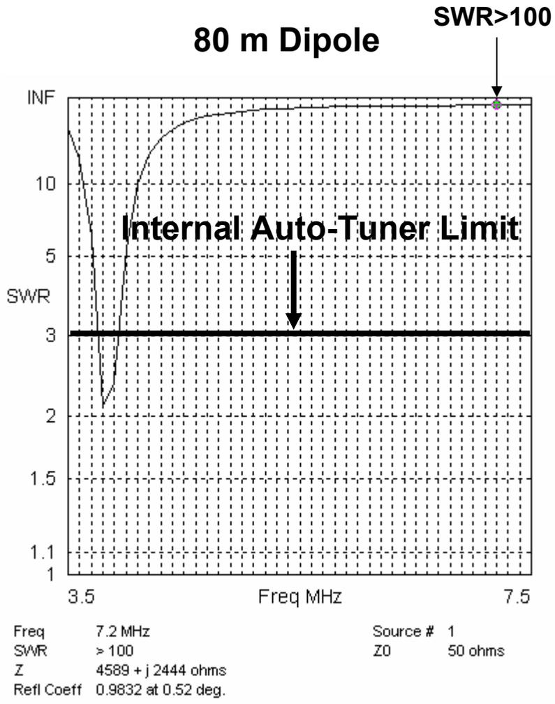
**Figure 13: SWR Plot of 75m NVIS Dipole**
