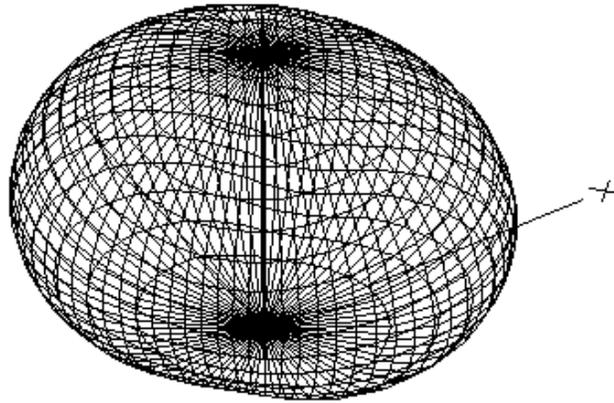
**Figure 10: Cross-Dipole Antenna Pattern at 75m**
