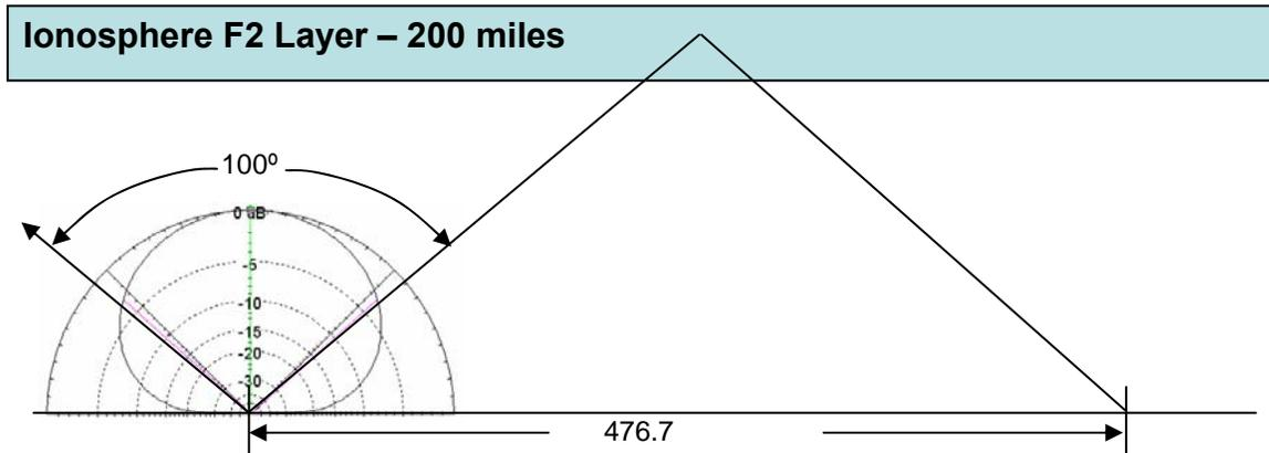
**Figure 1: Required NVIS Antenna Vertical Directivity Pattern**
