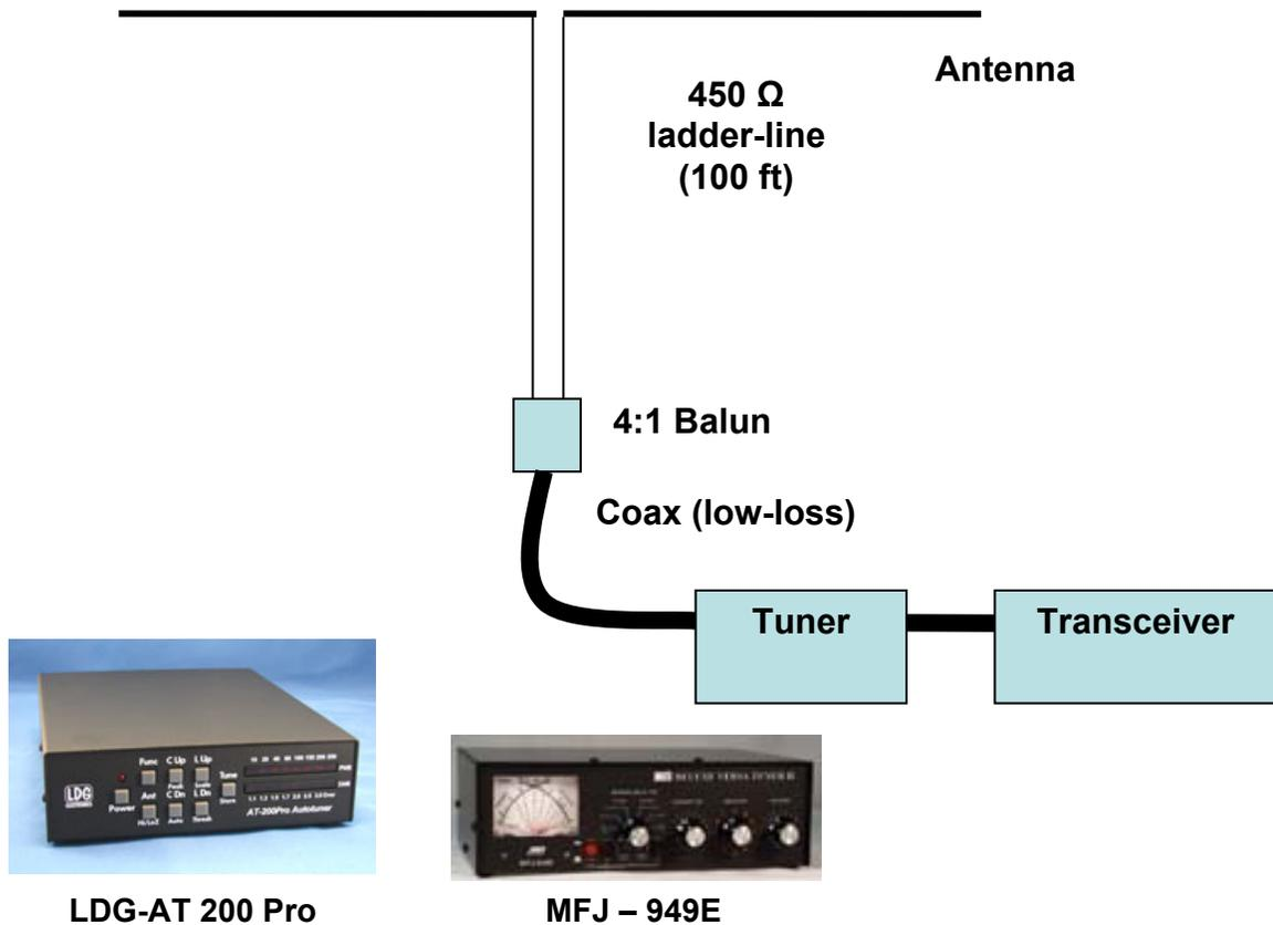
**Figure 16: Wiring Arrangement For A Tuner Located At Rig**
