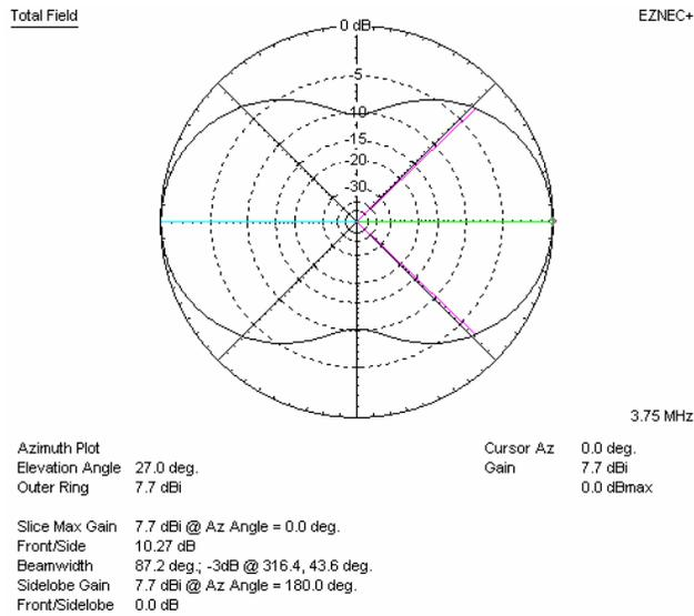
**Figure 5: Elevation Plot 75m Dipole at 1/2 Wavelength Height**
