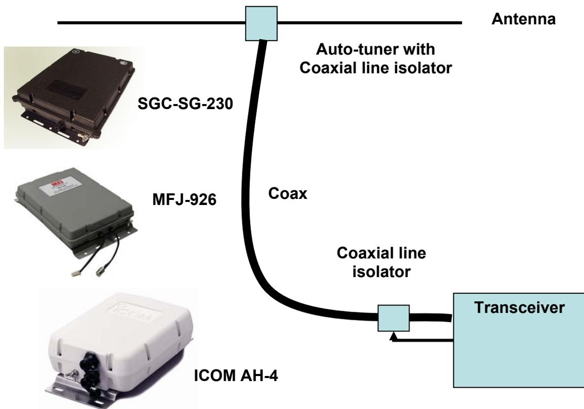
**Figure 17: Tuner At The Antenna**
