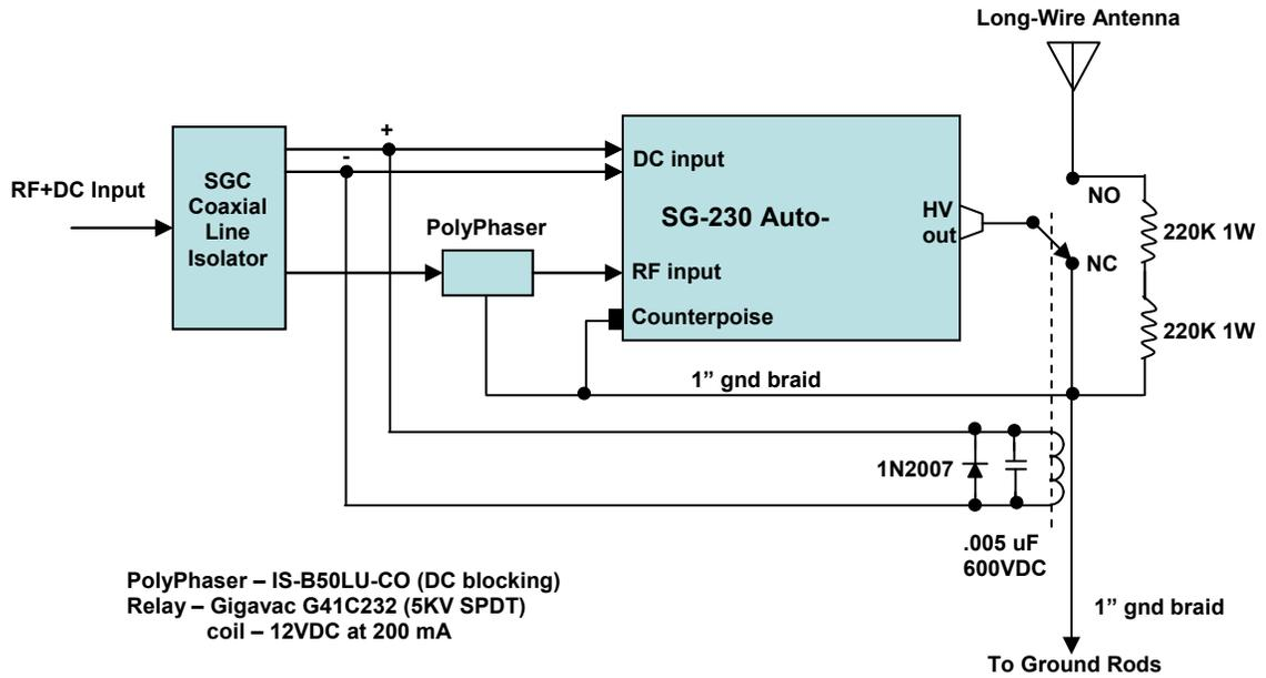
**Figure 18: Auto-Tuner Lightning Protection Circuitry**
